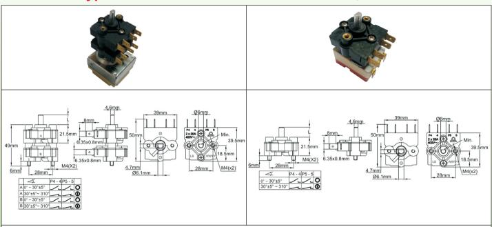
These on-off switches are designed to be added on thermostat shafts. They provide off position when the thermostat shaft is at the minimum position. They are available in single pole contact, two pole (one level) and three pole or four-pole contact (two levels).
